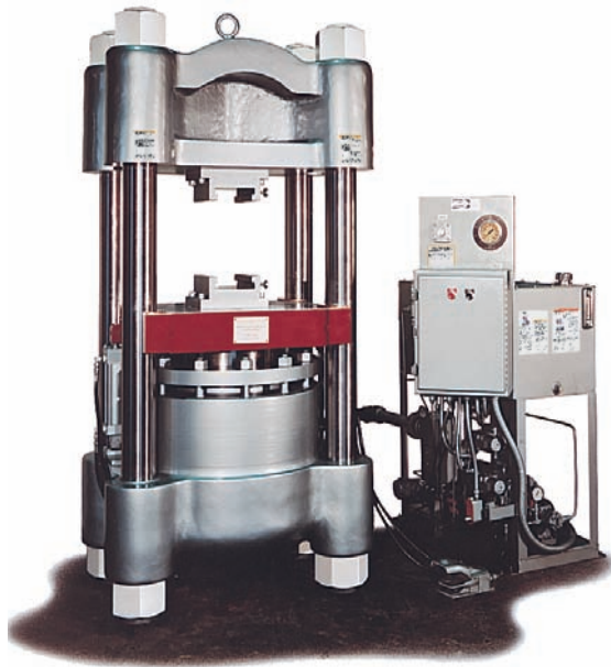
1500 Tonnes Hydraulic Swaging Machines Approximate weight 15.6t. Overall height 2.6m. Fast advance and retract speed. Automatic slow, precision swaging speed.
