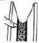
CORRUGATED GROOVES ACCELERATE WEAR OF WIRE ROPE
